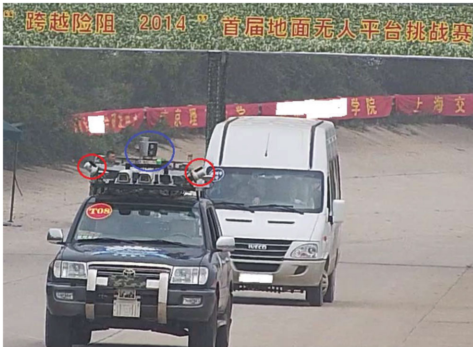
Figure 1. The proposed setup of 3-D LiDARs on our ALV platform: two compact HDL-32 LiDARs are mounted on the two sides of the vehicle top with a same fixed angle (labeled by a red circle); another HDL-64 LiDAR is upright equipped on the middle of the vehicle top for comparison (labeled by a blue circle). This vehicle won the champion in the “Overcome Danger 2014” ground unmanned vehicle challenge of China, the background is the challenge spot.
