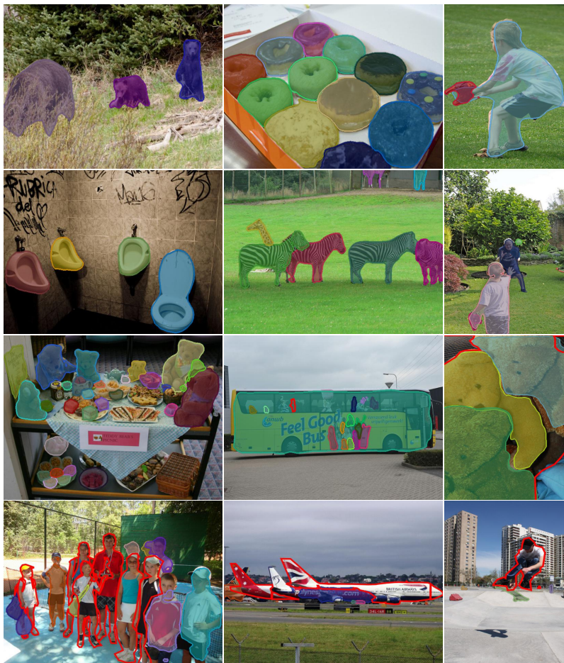
Fig. 4: SharpMask proposals with highest IoU to the ground truth on selected COCO images. Missed objects (no matching proposals with \text{IoU} > 0.5 ) are marked in red. The last row shows a number of failure cases.
