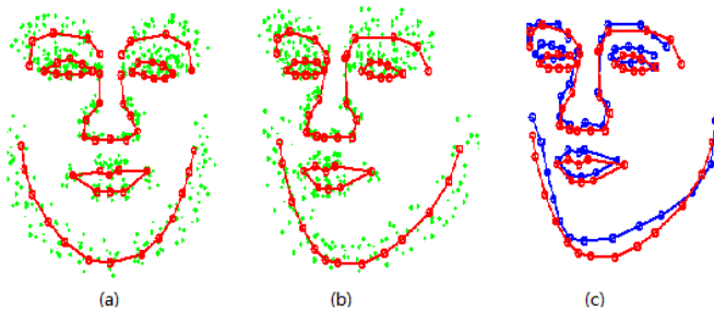
Fig. 1. A small experiment conducted with neighborhood-preserving estimation method: red and green dots represent the landmark points in testing and training shapes, blue dots represent the estimating landmarks, (a) testing shape and the shapes of the ten nearest samples for testing sample in frontal view; (b) the shapes of the testing sample and its ten nearest neighbors in non-frontal view; (c) the estimated shape with our method
